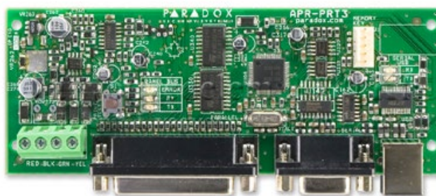
33.34 – Paradox APR-PRT3 integration and printer module
