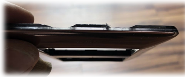
26. 27 – Frame cut out for air flow
