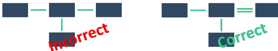
11. 12 - CAN bus, incorrect branch and solution with two cables
